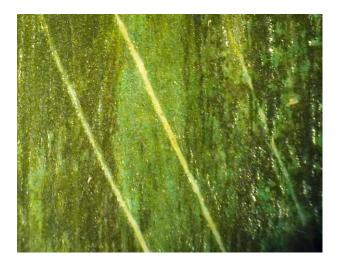
RMSS 5: This shows three unusual crevices running through the exposed ground layer, roughly parallel to each other. They appear to have been caused by the dragging of an implement across paint softened by solvent. There are no jagged edges, which rules out the possibility of a simple scratch or abrasion.
